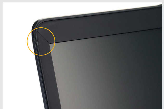
Medium crack on display frame.
