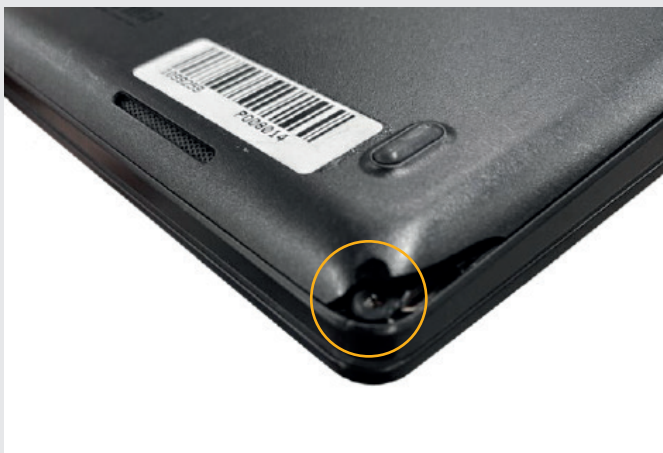
Housing damaged major, missing plastic part.
