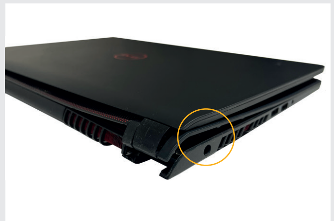
Housing with major damages.
