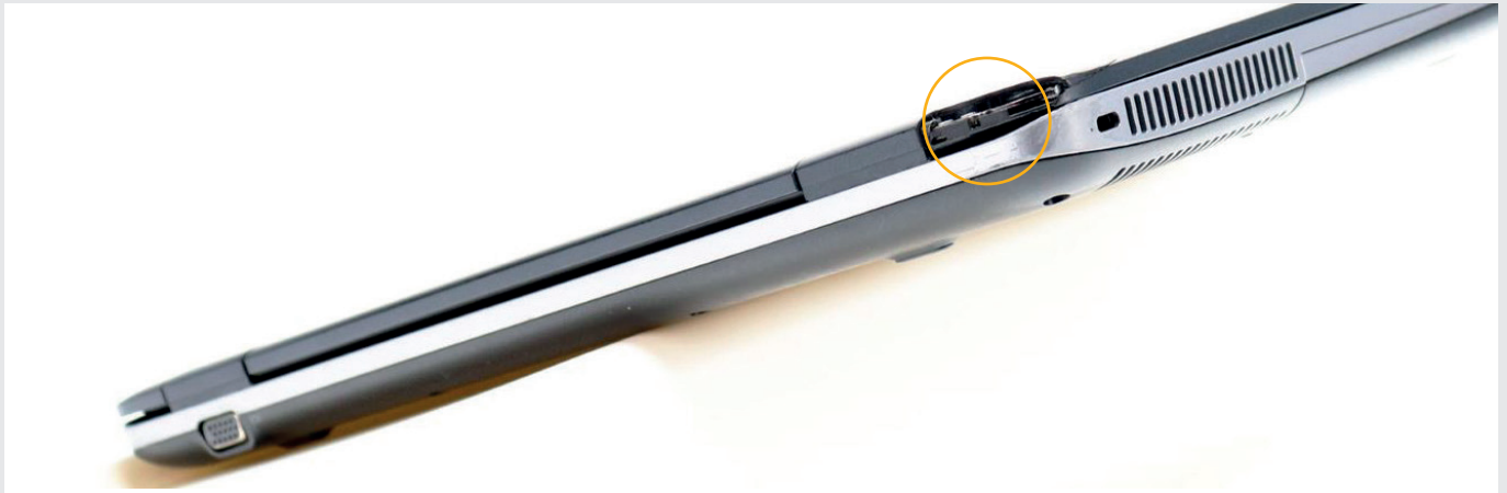
Housing damaged major, missing plastic part.
