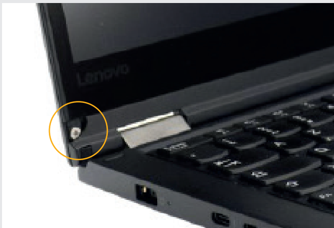
Display frame damaged major, parts missing.
